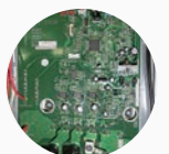
3 Sine-wave DC inverter control
